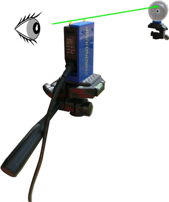
Figura 12.1: Alignment of the photocell
