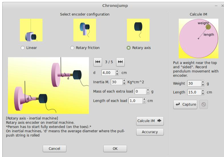
Figure 5.25: Parameters for calculating the IM
