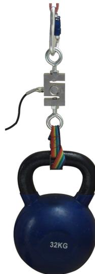
Figura 5.38: Force sensor calibration
